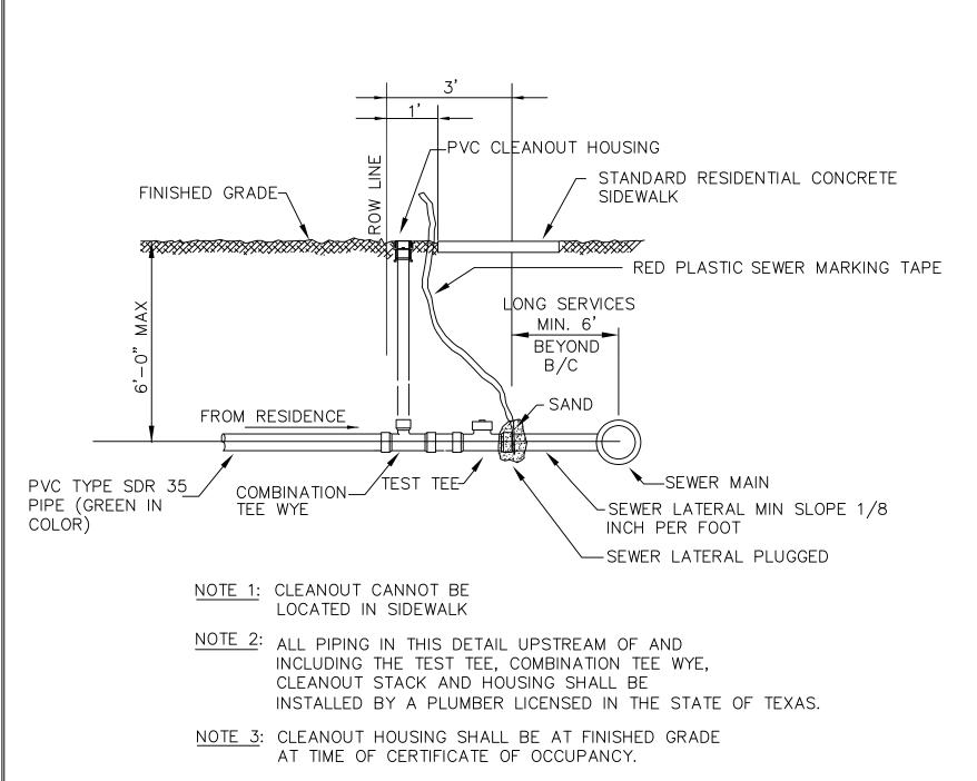
NOTE 4: SHOULD CLEANOUT BE LOCATED IN DRIVEWAY PAVING, THE CLEANOUT HOUSING SHALL BE DUCTILE IRON OR BRONZE.
