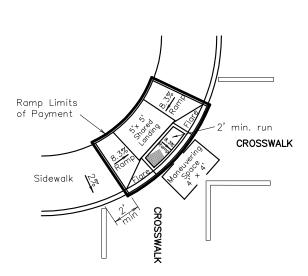
DIRECTIONAL RAMP WITHIN RADIUS (Sidewalk set back from curb)
