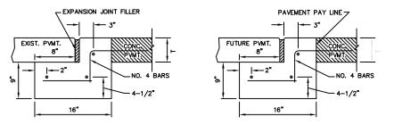
PAVEMENT BARS TO BE BENT DOWN INTO HEADER. HEADER AND PAVEMENT TO BE MONOLITHIC.
